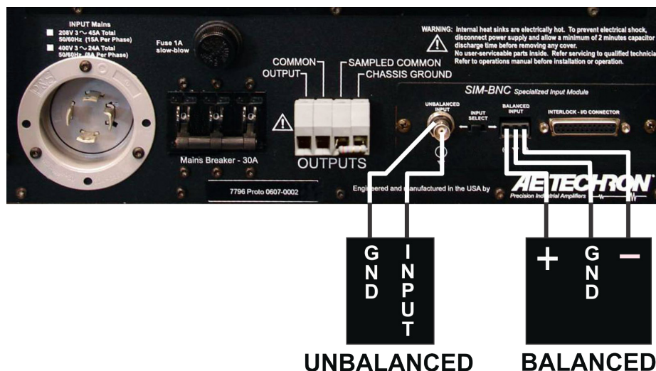
Figure 2.4 – Wiring for Unbalanced or Balanced Input Connector
