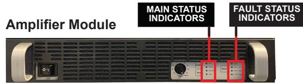
Figure 3.7 – Amplifier Module Status Indicators
