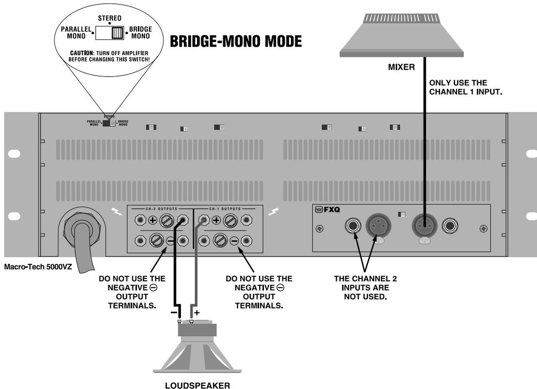
Fig. 3.5 Bridge-Mono Wiring
