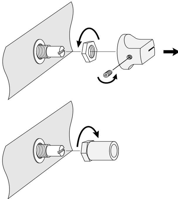
*Fig. 8.2 Installing a Level Control Shaft Lock*
