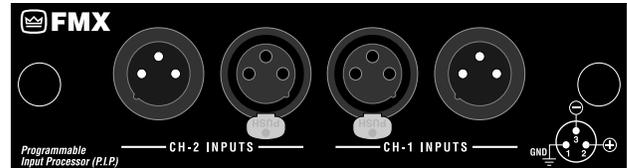
**P.I.P.-FMX** facilitates “daisy-chaining” balanced amplifier inputs. Female to male three-pin XLR connectors are used to passively bridge the inputs.
