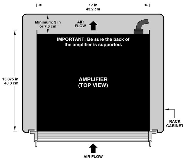
Fig. 3.2 Top View of a Rack-Mounted Unit
