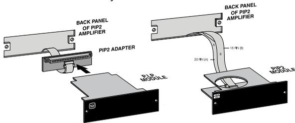
Fig. 8.1 Installing a *PIP* or *PIP2* Module
