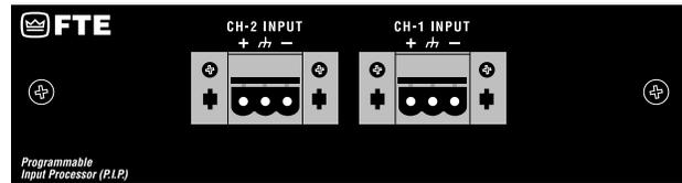
**P.I.P.-FTE** uses balanced 1:1 transformers to isolate the amplifier from the input signal. It also includes 12 dB/octave RFI filters, 18 dB/octave high pass filters, and 6 dB/octave 3 kHz shelving networks for “constant-directivity” horn equalization. Screw terminal plugs are provided for input.
