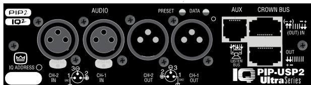
**IQ-PIP-USP2** is an IQ2-series component. This means it supports Crown’s UCODE protocol and requires an IQ System with an IQ2-compatible IQ interface. UCODE (universal code) enables users and third parties to develop custom software objects to control and monitor IQ2-compatible components like the IQ-PIP-USP2.
