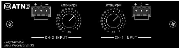
**P.I.P.-ATNB** uses balanced 1:1 transformers to isolate the amplifier from the input signal. It also includes 12 dB/octave RFI filters, variable 18 dB/octave high-pass filters, and 6 dB/octave 3 kHz shelving networks for “constant-directivity” horn equalization. The module also includes a calibrated 21-step precision attenuator for each channel. Screw terminal plugs are provided for input.
