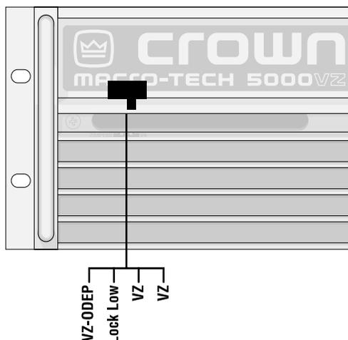
Fig. 4.4 Channel 1 VZ Mode Switch (Behind Filter)
