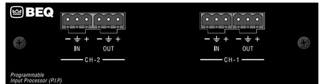
**P.I.P.-BEQ** is a two-channel module providing equalization for BOSE® loudspeakers. For example, the P.I.P.-BEQ can be used in place of a BOSE 102 controller. Screw terminal plugs provide balanced connections. Each input channel has an output from the PIP that can be independently configured for output with no processing, loudspeaker equalization or loudspeaker equalization with bass-cut.
