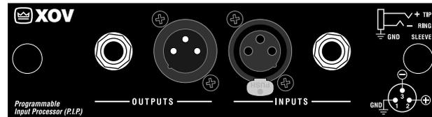
**P.I.P.-XOV** is a versatile 18 dB/octave mono crossover/filter with blamping and triamping capabilities
