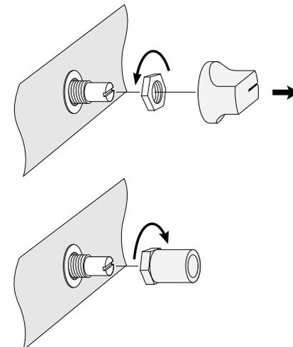
Figure 5.4 Installing a Level Control Shaft Lock
