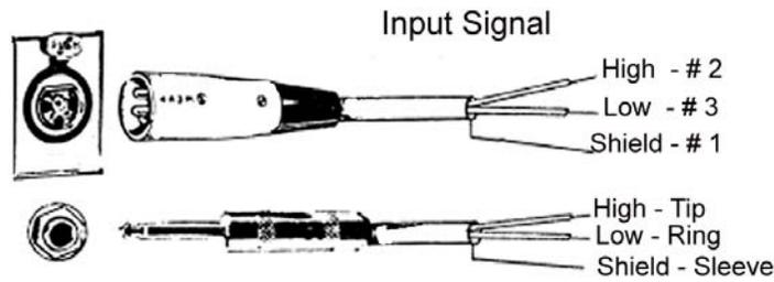
Figure 1. Balanced Input Connections\*
