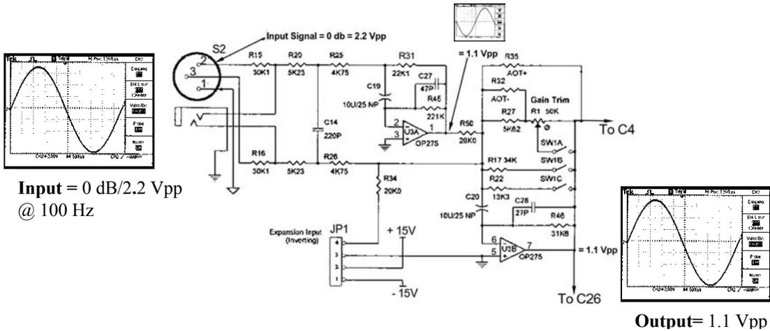
The integrated circuit, U3, provides several functions. U3A is used as an input buffer amplifier which isolates the source signal from deterioration caused by the user selectable DIP switches, SW1A.,B,AND C. The resultant gain of U3B will vary depending upon which DIP switches are enabled. The final composite signal on pin 7, U3B, is sent to coupling capacitors C4 and C26 which provide access to the low and high frequency processing circuits, respectfully.
