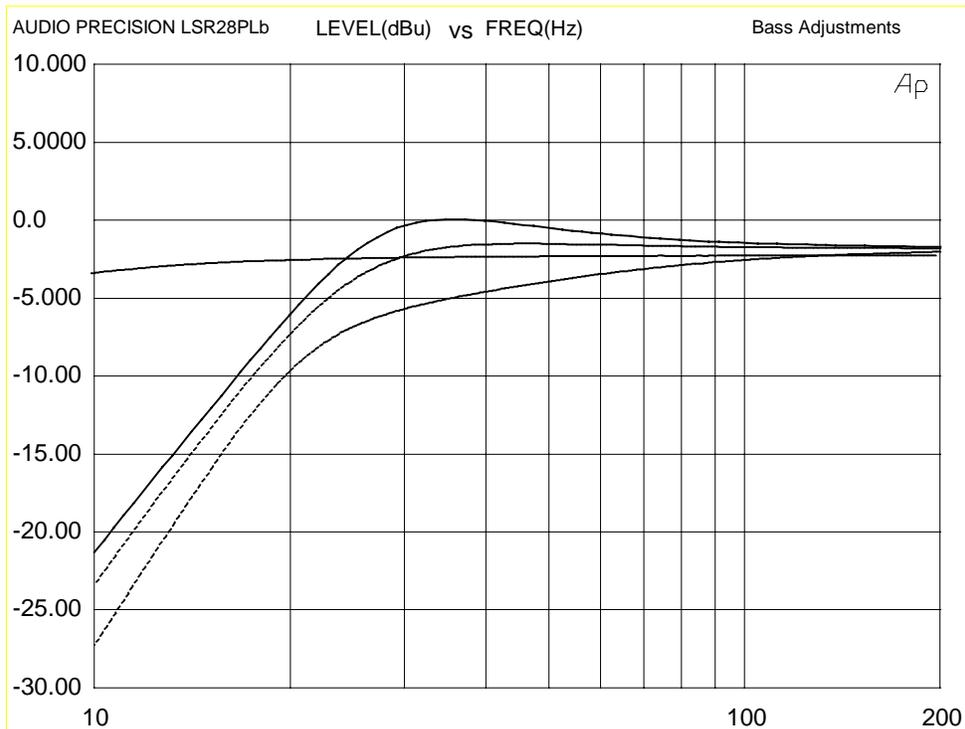
The response at any point along the signal path relies on an accurate frequency response characteristic from preceding stages. The curves in the figure allow ready identification of a stage, which is causing frequency response errors. An inaccuracy in a single section can result in gross inaccuracies in the overall response result.
