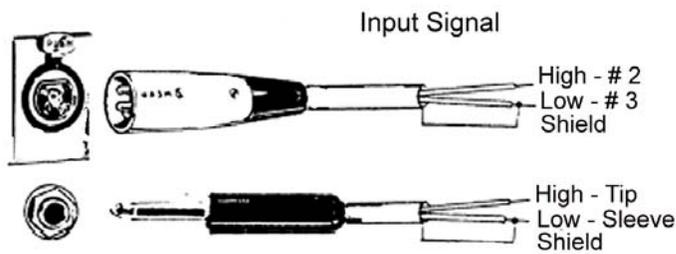
Figure 2. Unbalanced input Connections\*
