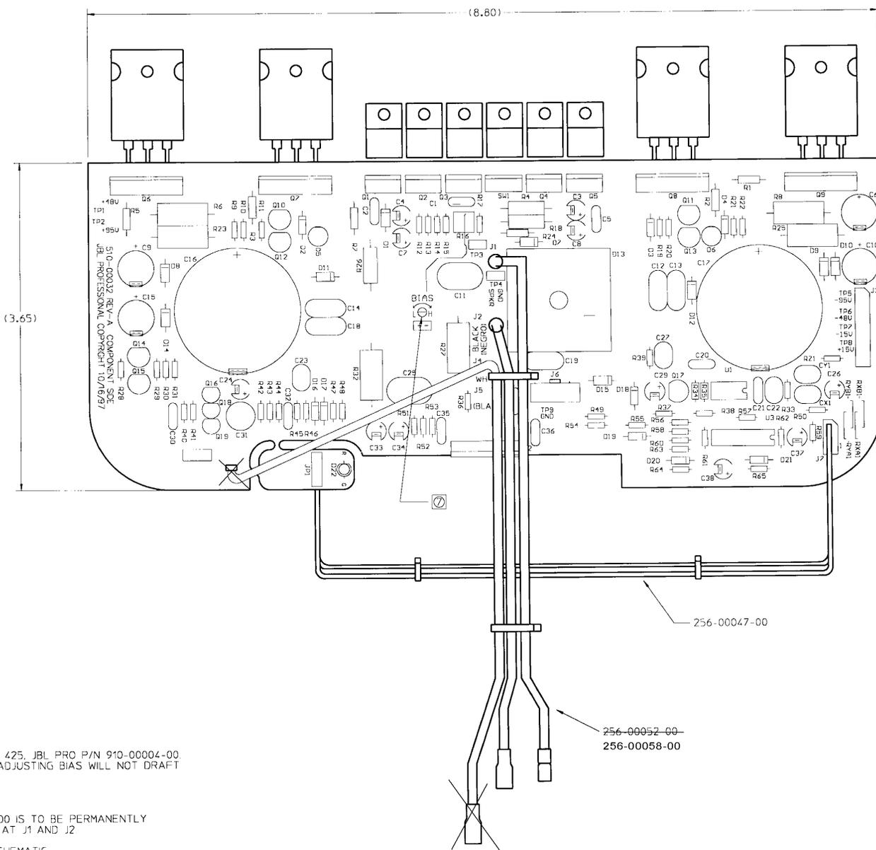
USE 0.00005 GRAMS OF LOCTITE 425, JBL PRO P/N 910-00004-00 OR EQUIVALENT ON R17 AFTER ADJUSTING BIAS WILL NOT DRAFT WITH VIBRATION
