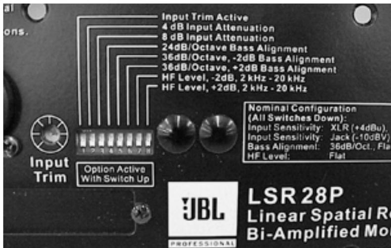
Located on the right of the Neutrik connector but before the power switch, is a bank of switches that are accessible with the use of a pen or a very small screwdriver. These are the DIP switches.
