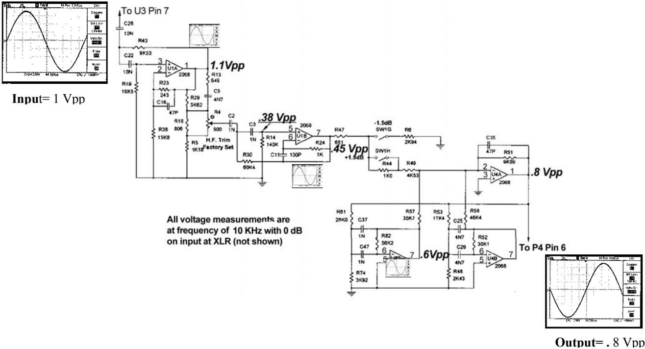
The circuit, shown above, is used for the high frequency processing of the input signal. Physically, it is located on the input circuit board. Its purpose is to actively filter out or attenuate the low frequency component from the composite signal leaving only the high frequencies to be contoured by the user and, eventually, sent to power amplifier for final amplification.
