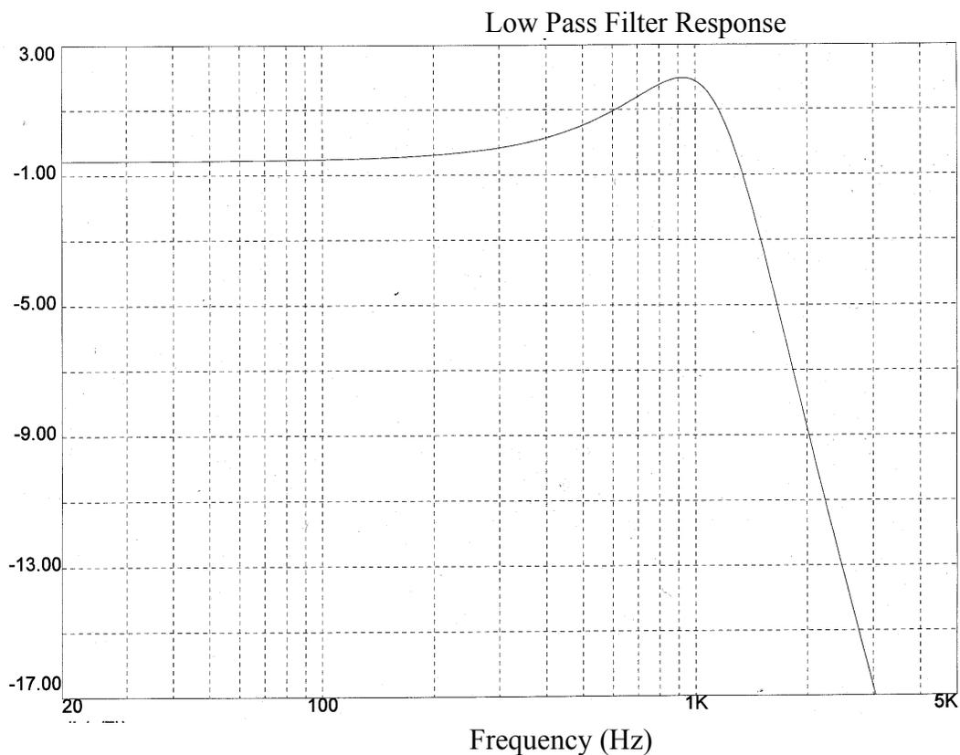
This is a low-pass filter with the half power point at 1500 Hz. If the response is incorrect check the values of RZ1, R33, CY1, CX1 and C22. If these values are okay, check the values of C23, C24, R48 and R42.
