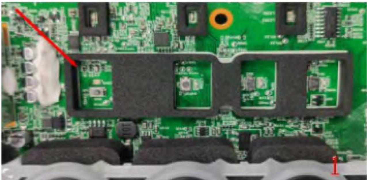
Step 7: Confirm whether the tact switch of BT button is damaged.
