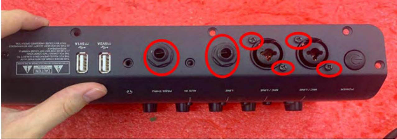
Step 4: Remove the 6 screws holding Main PCBA to amp chassis.
