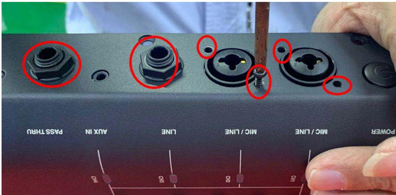
Step 15: Use locktight to keep the screws from backing out from vibration.
