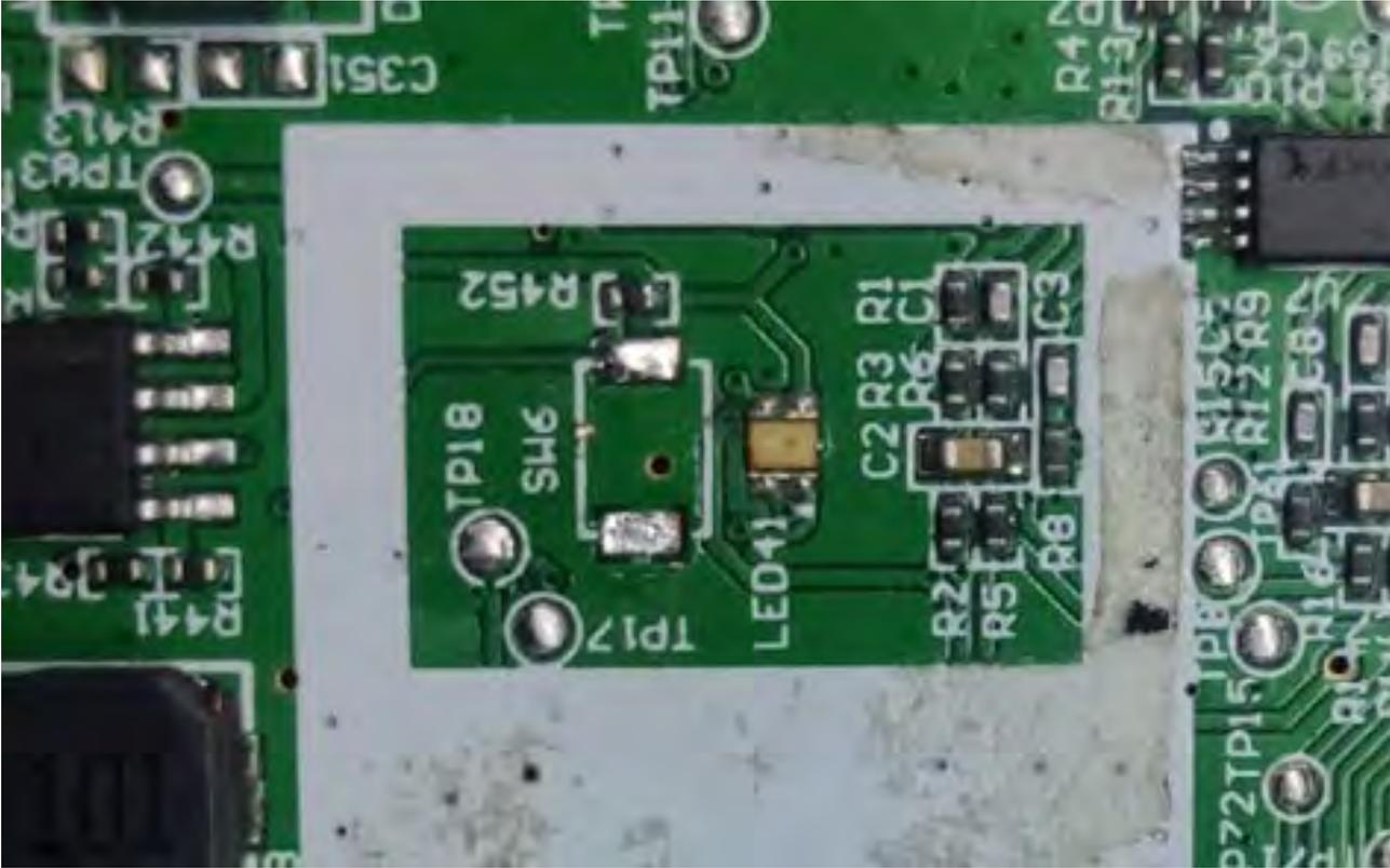
3) Place the tact switch according to positioning line, and solder switch to PCB.
