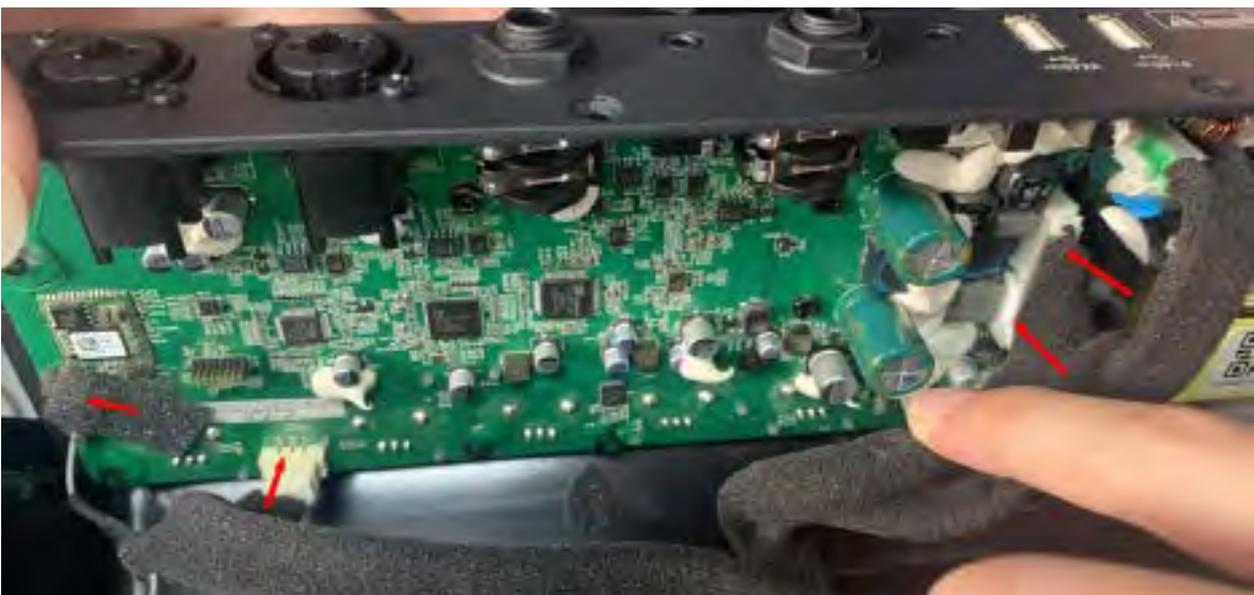
Step 17: Position the Amp Assy back into place with the Compact SPK, and tighten the screws in the following sequence. You are now ready for final testing to verify correct operation.
