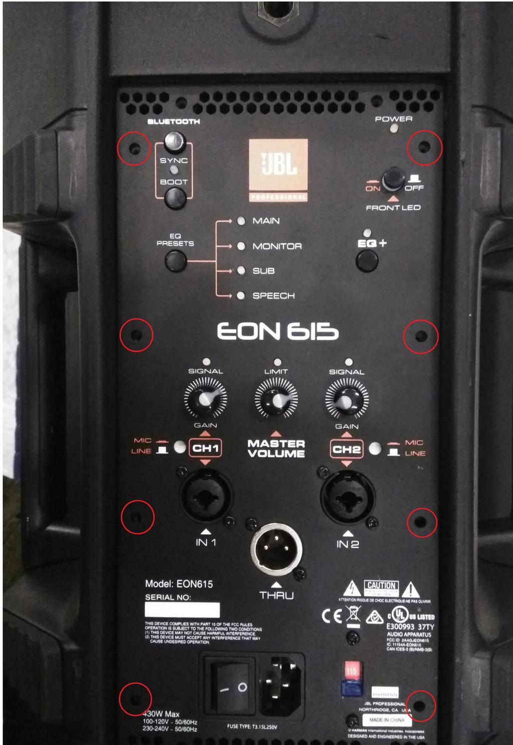
Figure 1. Amplifier Module Cover
