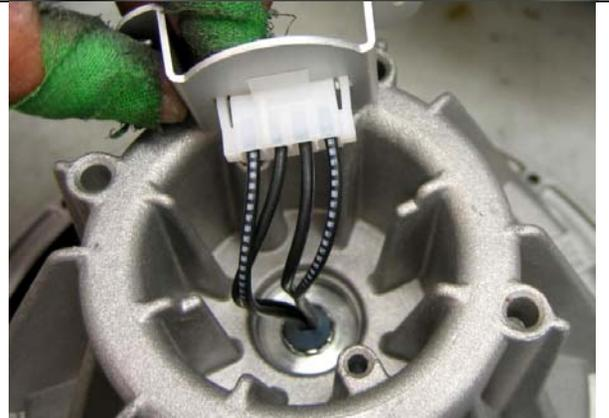
**Photo #3. Fasten the terminal cup with the 2 screws provided.** Make sure the JBL logo on the cup is in the same orientation as the logo in the frame.
