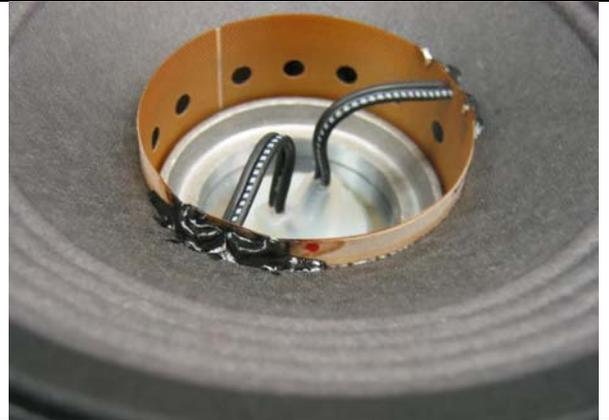
**Photo #2. Correctly installed wires / terminal cup assy.** Notice the wire pairs remain together, and the white striped wires are towards the outside of the housing. Ensure the contacts are fully inserted into the housing until they click into place. Tug on each wire after inserting to make sure each is positively locked into position.
