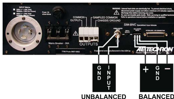
Figure 2.11 – Wiring for unbalanced or balanced input connector
