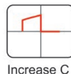
Figure 5.16 – Square Wave Showing an Increase in C is Required
