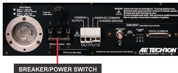
Figure 5.1 – Amplifier Module's Breaker/Power Switch Location
