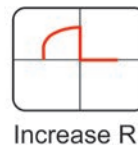
Figure 5.15 – Square Wave Showing an Increase in R is Required
