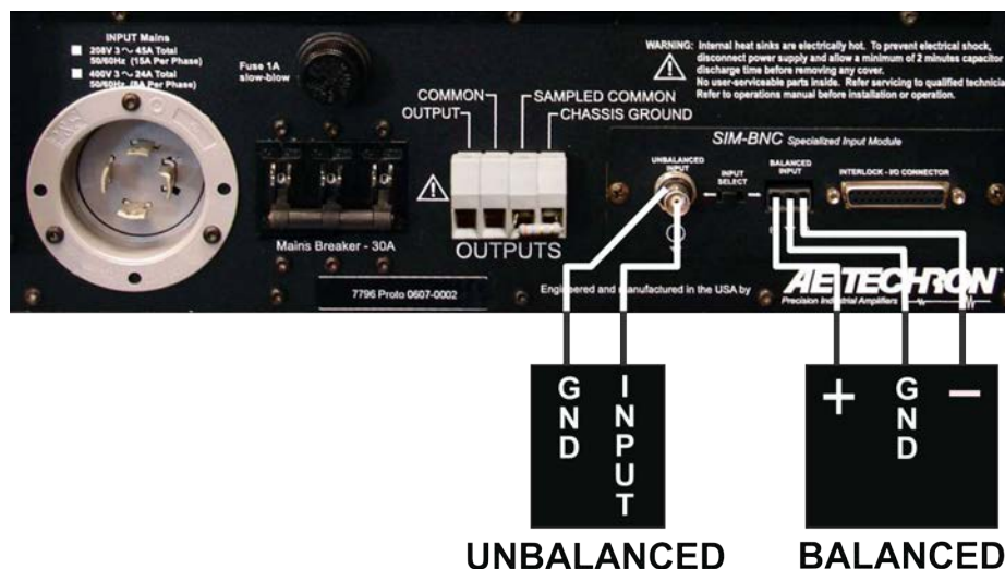
Figure 2.4 – Wiring for Unbalanced or Balanced Input Connector
