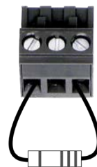
Figure 5.21 – Terminating the Amplifier Input
