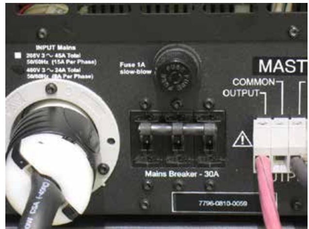
Figure 6.1 – Location of Back-Panel Circuit Breakers and Fuse F1
