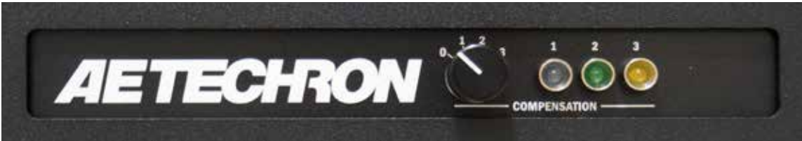
Figure 3.3 – 4301 Compensation Control Panel
