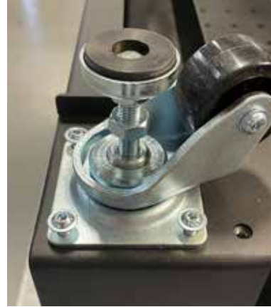
Figure 2.3 – Leveling pads on Cabinet Wheels
