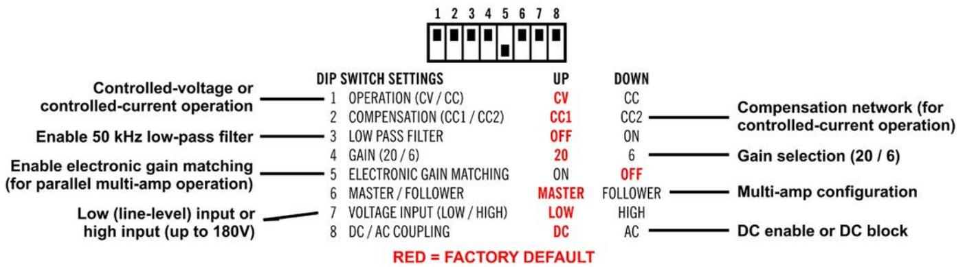
Figure 5.1 – DIP Switch Settings and Descriptions
