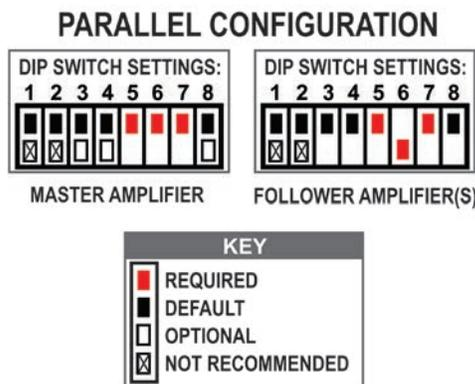
Figure 6.24 – DIP Switch Settings for Parallel Configuration
