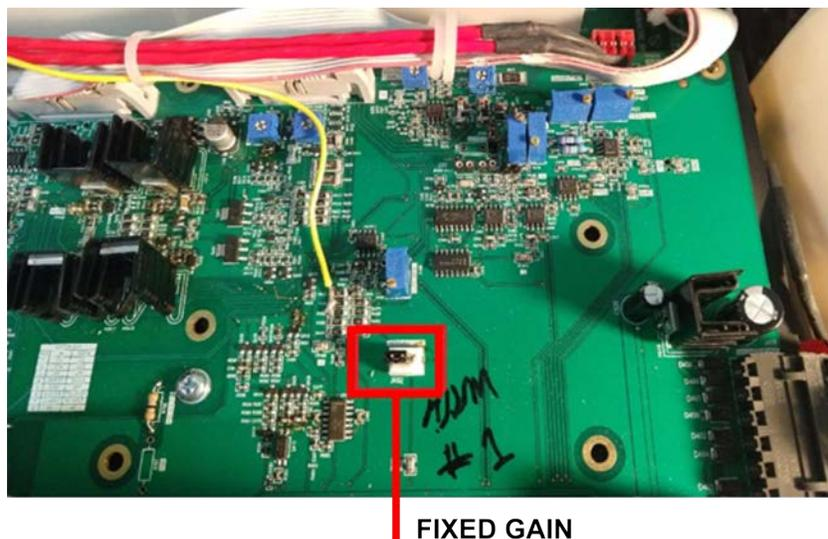
Figure 5.4 – Configure for Fixed or Variable Gain
