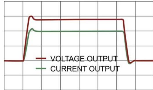
Figure 6.13 – Input to Output Comparison, Controlled-Voltage Operation
