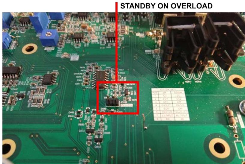
Figure 5.5 – Configure for Standby (Fault Mode) on Overload
