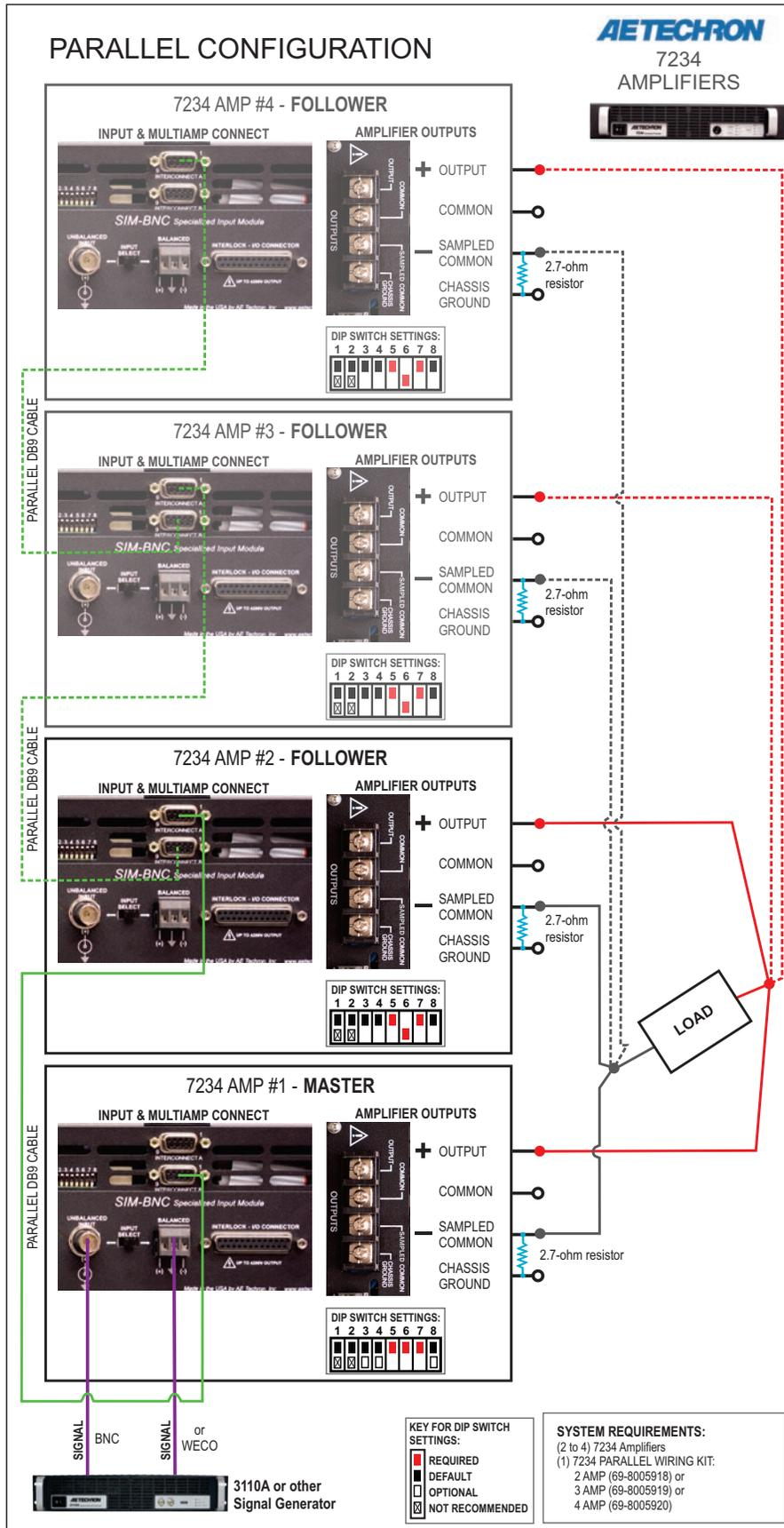
Figure 6.25 – Configuration and Wiring for Parallel Operation
