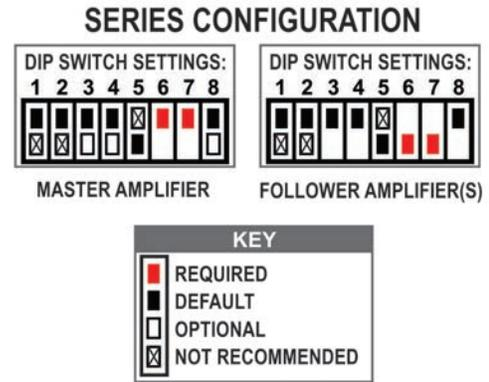
Figure 6.26 – DIP Switch Settings for Series Configuration
