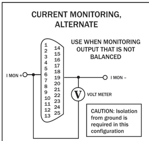
Figure 6.11 – Remote Current Monitoring, Alternate Method
