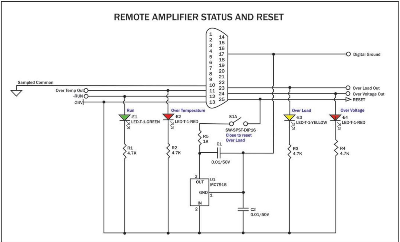
Figure 6.8 – Remote Status and Reset Schematic
