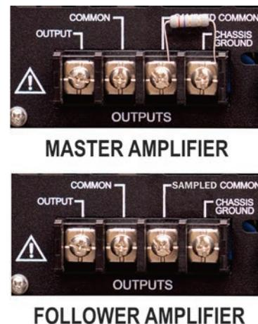
Figure 6.29 – Remove the 2.7-ohm resistor from Follower amplifiers
