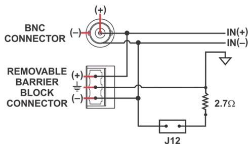
Figure 6.28 – SIM-BNC-OPTOC input connectors' internal wiring
