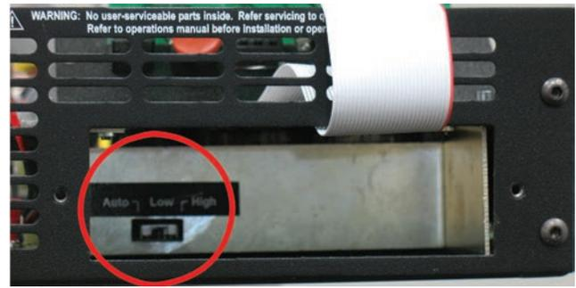
Figure 5.12 – Bi-Level Power Switch Location
