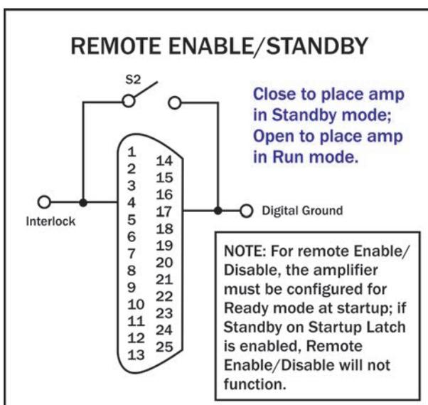
Figure 6.9 – Remote Enable/Standby
