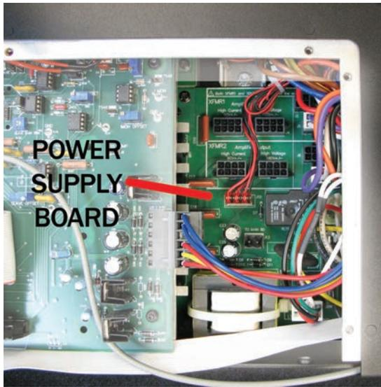
Figure 5.8 – Accessing the Power Supply Board
