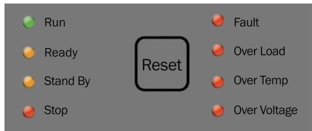
Figure 4.4 – Main Status and Fault Status Indicators
