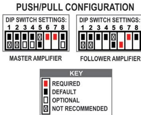
Figure 6.22 – DIP Switch Settings for Push/Pull Configuration
