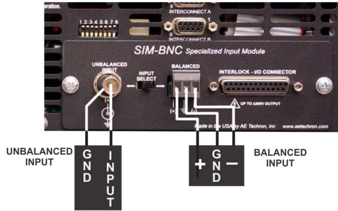
Figure 3.3 – Wiring for Unbalanced or Balanced Input Connector
