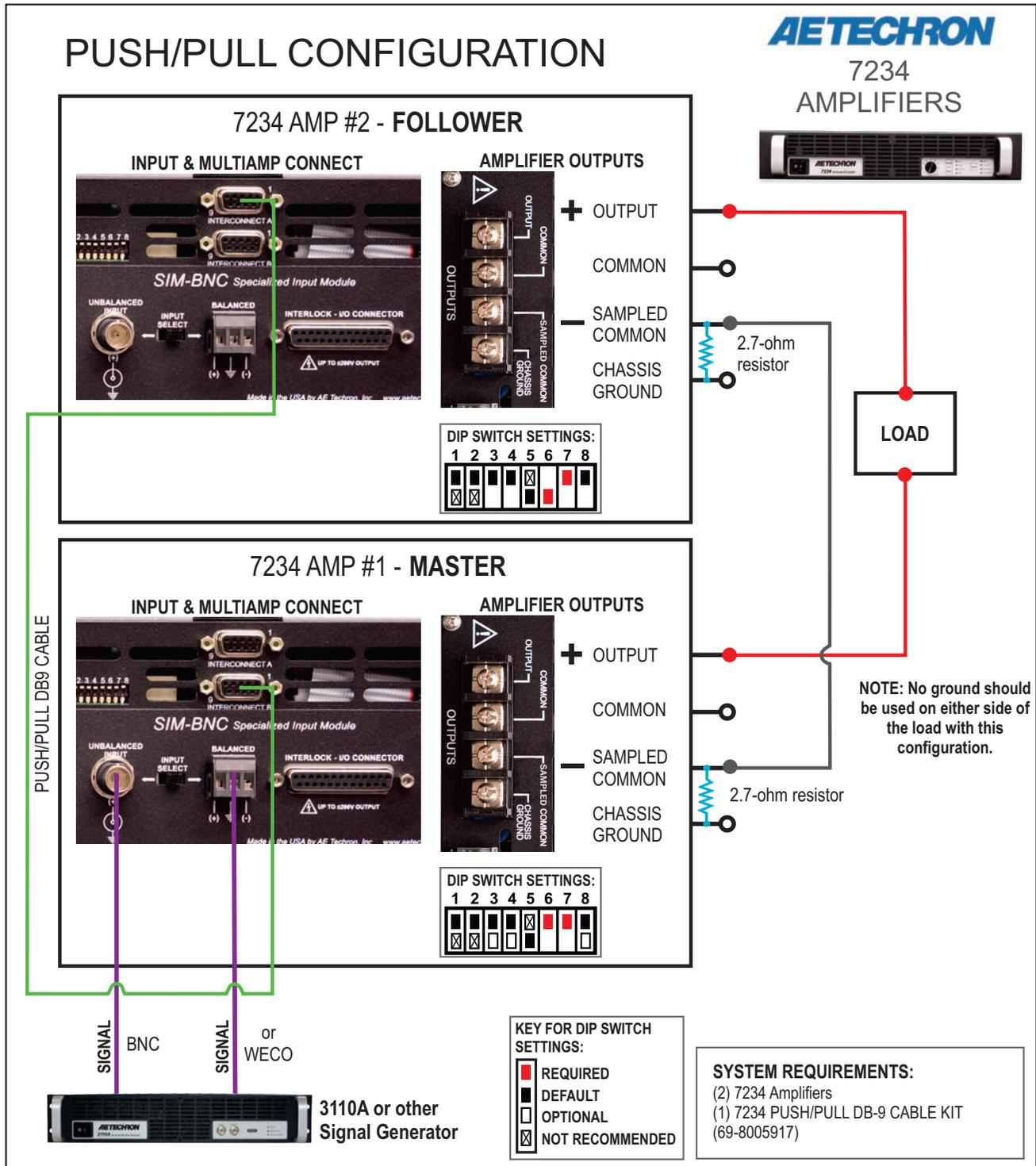
Figure 6.23 – Configuration and Wiring for Push/Pull Operation
