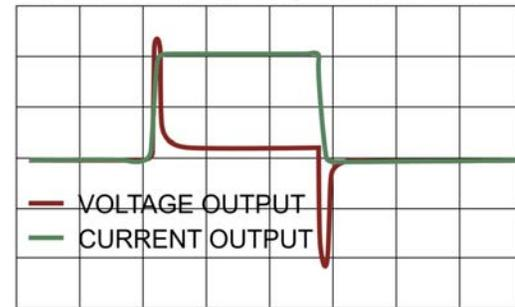
Figure 6.14 – Input to Output Comparison, Controlled-Current Operation
